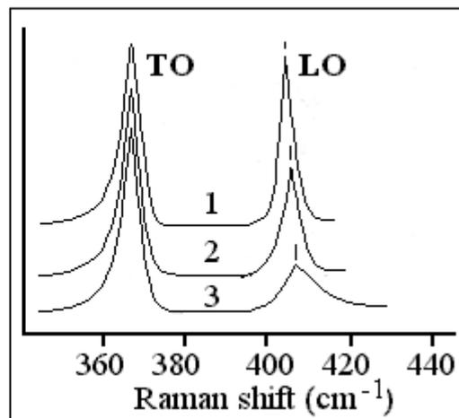
Fig.4. Evolution of LO lattice phonon energy with N concentration in ordered GaP:N according to Raman scattering at 300K. Excitation by Ar<sup>+</sup>-laser at 514 nm. Concentration of N grows in 3 orders from 1 to 3 (app.  $10^{19}$  N in cubic cm).
