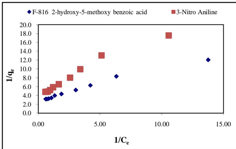
Fig. 2 : Langmuir adsorption isotherm system : F-816\_  $Co^{2+}$  at 298K
