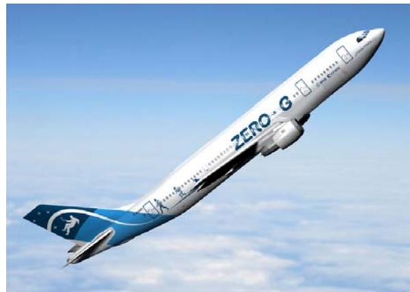
**Fig. 2** The Airbus A300 in pull-up (Photo: Novespace)
