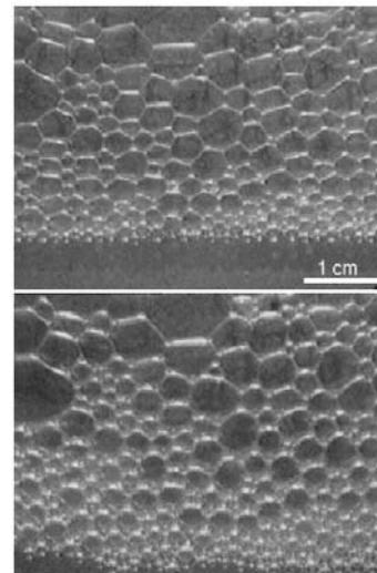
**Fig. 8** Foam in 1g (top: drainage) and 0g (bottom: no drainage) (Image: GRASP)<sup>18</sup>
