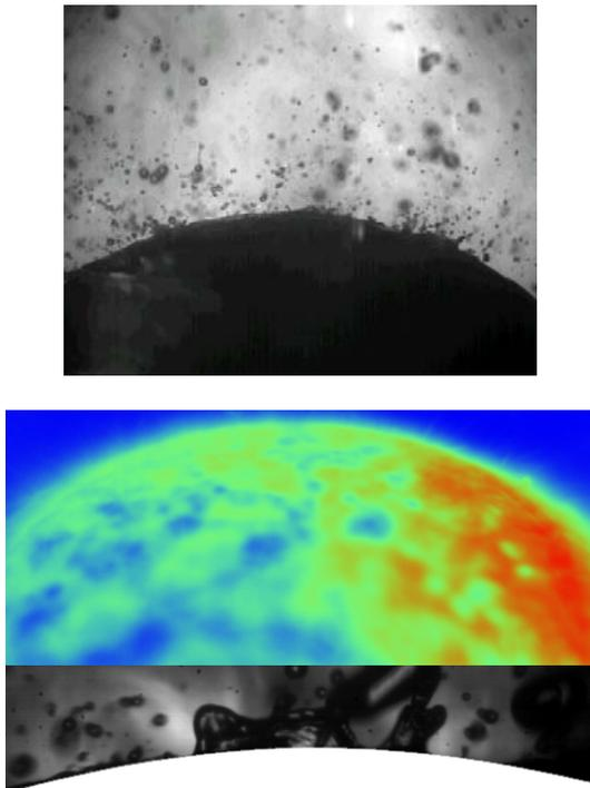
**Fig. 4** Spray impact on a heated target: high-speed, IR and high-res. views (Images: DOLFIN scientific team)<sup>14</sup>
