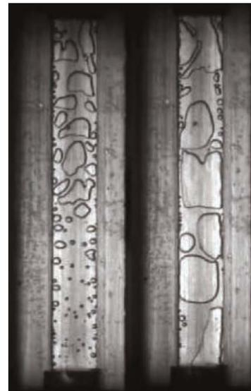
**Fig. 7** Flow boiling in a microchannel (upward flow): left: 2g, right: 0g (Image: IUSTI)<sup>17</sup>
