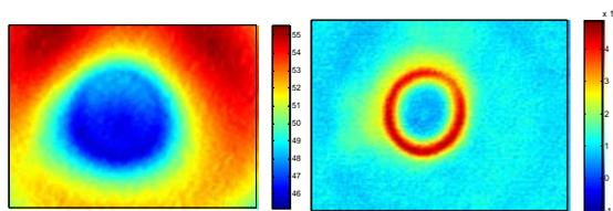
**Fig. 5** Measured wall temperature and calculated heat flux under a single vapour bubble (Images: TU Darmstadt)<sup>15</sup>
