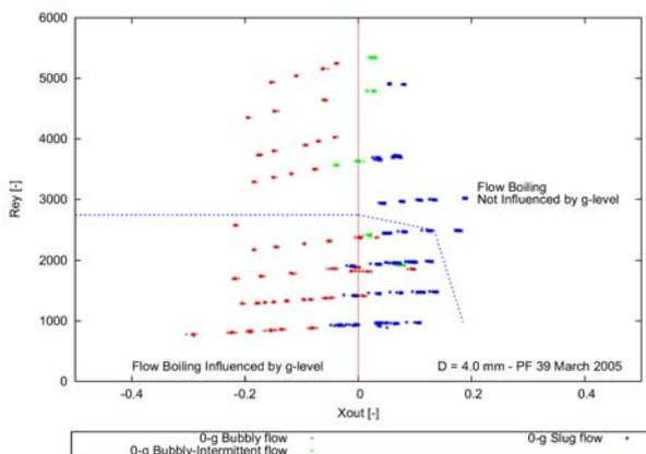
**Fig. 6** Threshold map for test section of diameter 4 mm (Image: ENEA)<sup>16</sup>
