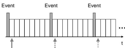
**Figure 1:** Segmented spiral event-related fMRI. After each event one segment of k-space (spiral interleaf) is acquired to attain high temporal resolution. The arrows denote the acquisition of the first (solid), the second (dashed) and the third (dotted) k-space interleaf of the first image of the time series.
