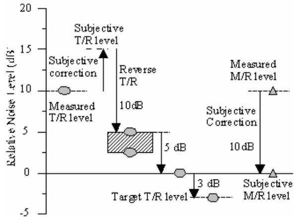
**Figure 6: Balanced Noise Source Concept**
