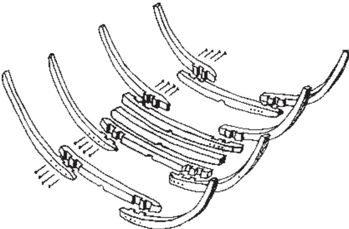
FIG. 5 – Presumable position of the master frames of the SJB2 wreck.
